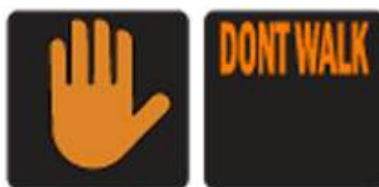
A fixed hand or fixed DON'T WALK sign (fixed means that the DON'T WALK signal is not flashing or counting down)
